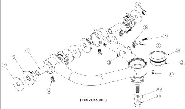
Torque M14 nut to 95 ft/lbs. w/ red loctite
